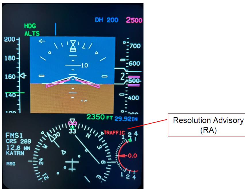
Figure 6 – Example of how an RA appears to pilots on an aircraft primary flight display (Source: TCAS Manufacturer Collins Aerospace through the NTSB)
