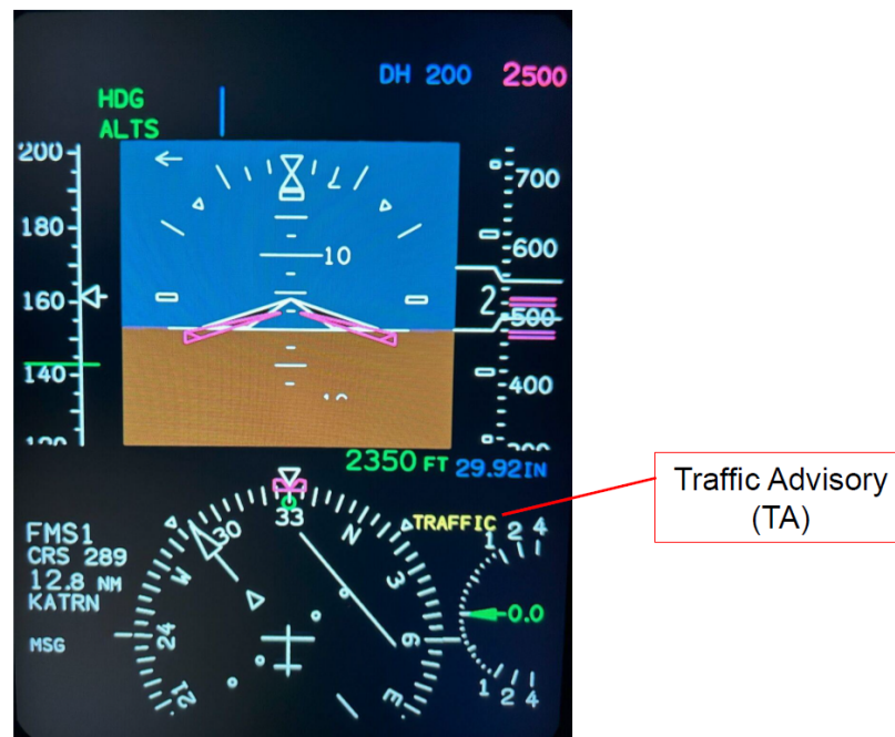
Figure 4 – Example of how a TA appears to pilots on an aircraft primary flight display (Source: TCAS Manufacturer Collins Aerospace through the NTSB)
