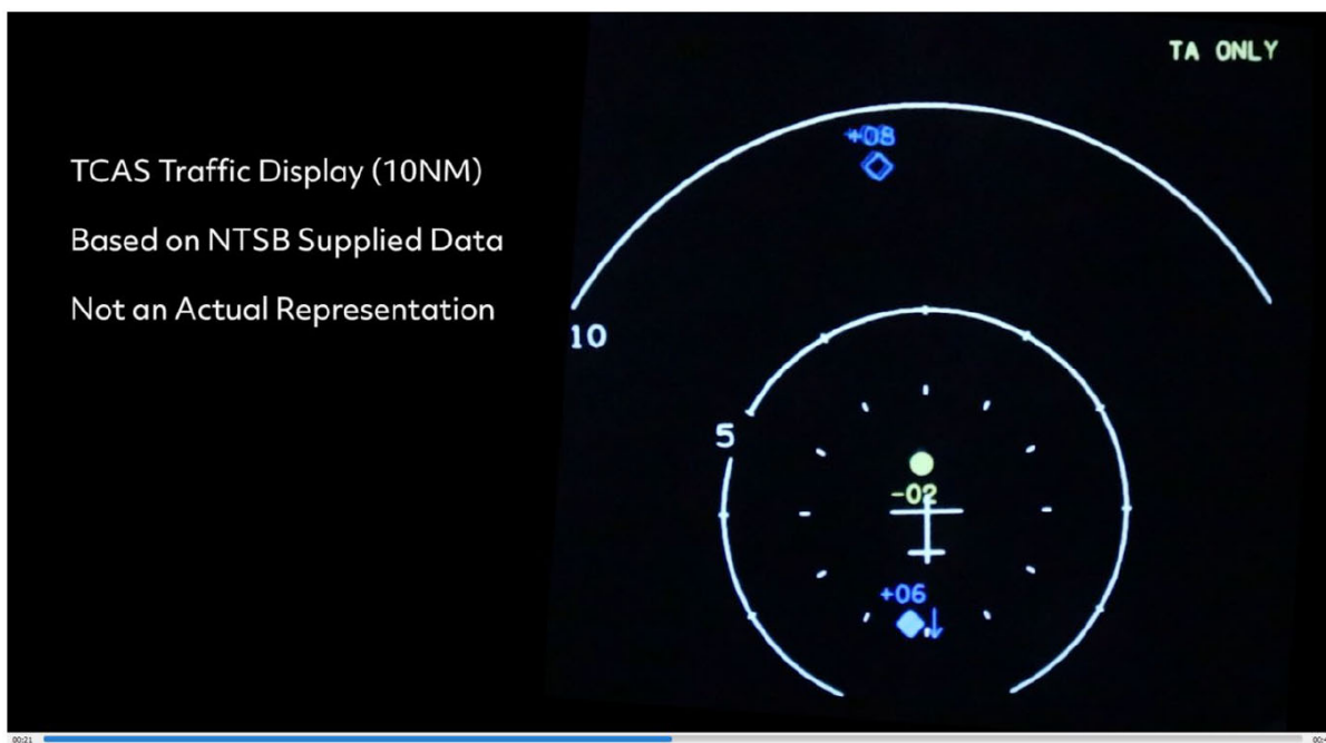
Figure 12 – Simulated TCAS Display Showing a Display Similar to What Would have been Displayed in the Subject Airplane approximately 20 Seconds Before the Collision, Showing the Helicopter as well as its relative Position and Altitude in Yellow (Source: NTSB Airplane TCAS Specialist Study, Inv. No. DCA25MA108)
