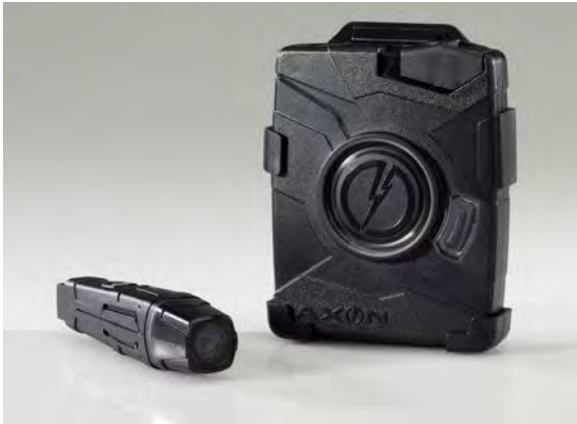
AXON Flex DVR and Controller: The DVR's multiple mounting options record the officer's POV.
